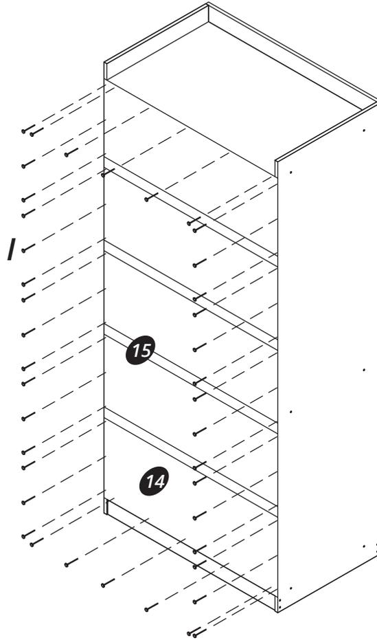
*Connect all the parts (14) joining with the part (15) and the hardware (I).*
