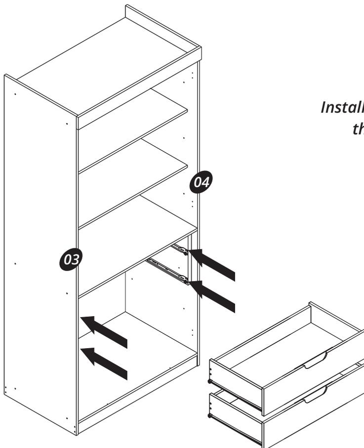
*Install the drawer fitting it into the slides fixed on the side of parts (03) and (04).*
