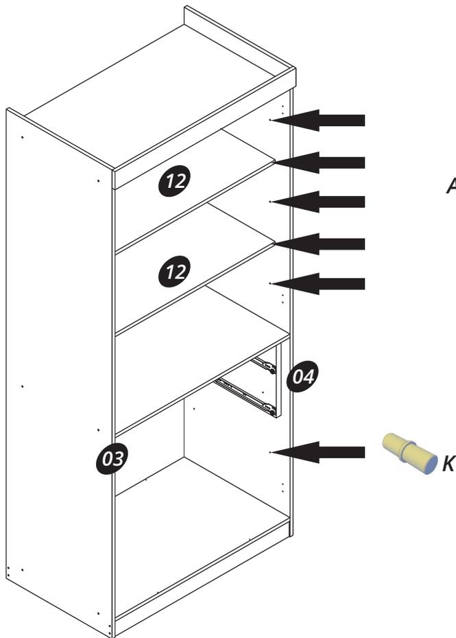
*Apply the hardware (K) into the part (03) and the part (04) to support the part (12).*
