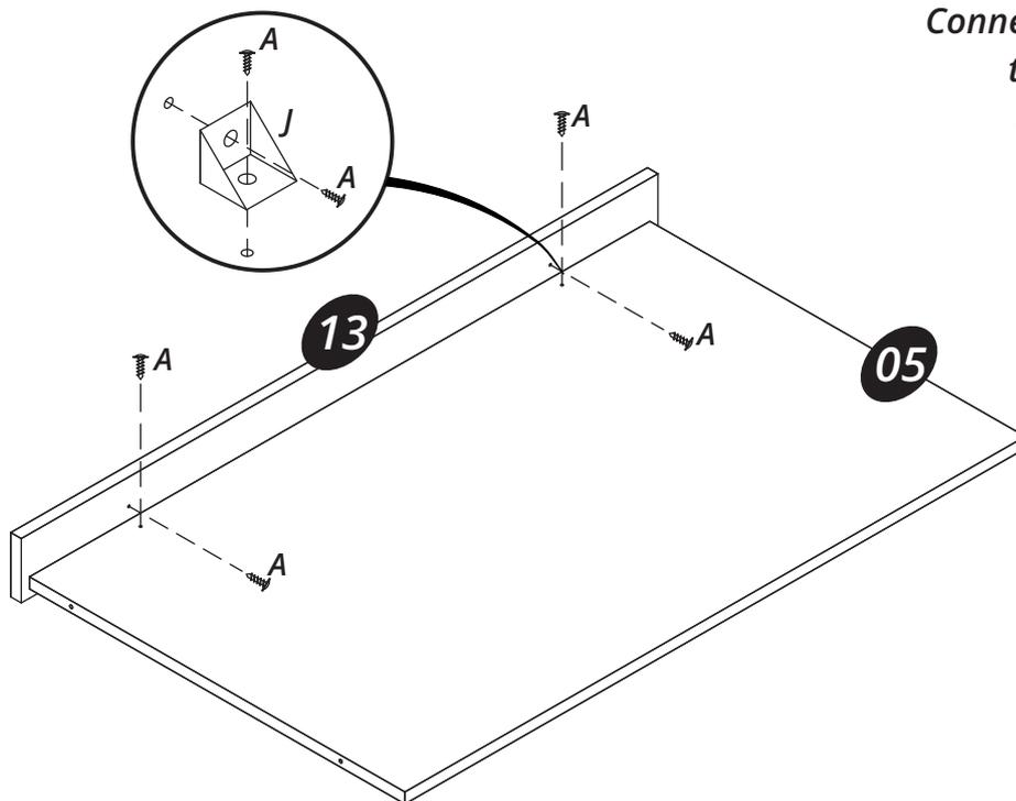
Connect the part (13) onto the part (05) with the hardware (J) and the hardware (A).
